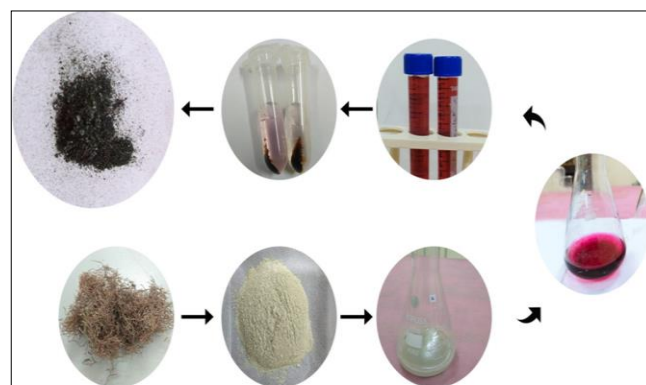
Fig 1: Process for synthesis of Manganese nanoparticle using aqueous extract of A. fragilissima
